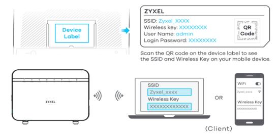
The SSID and Wireless Key are on the device label.
